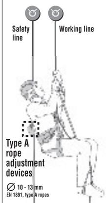
Type A rope adjustment devices
